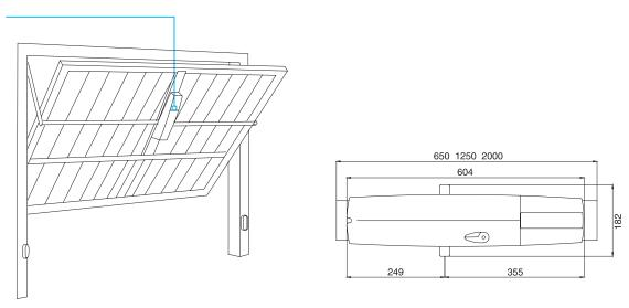
For protruding and non-protruding up-and-over doors of up to 9 m² (up to 14 m² using 2 motors), and jointed doors.
