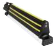
Sensitive safety edge with 8.2KΩ resistive contact, complying with UNI EN 12978, fitted onto an aluminium profile. L=170 cm.
