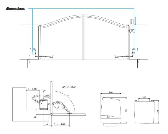
${\bf NB.}$  Angle ß to be kept between 30° and 120° to achieve optimum release; otherwise consider using the ARMAX arm
